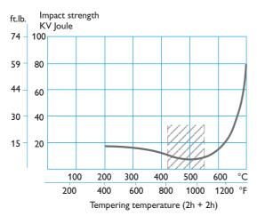
Tempering within the range 425–550°C (800–1020°F) is normally not recommended due to the reduction in toughness properties.
